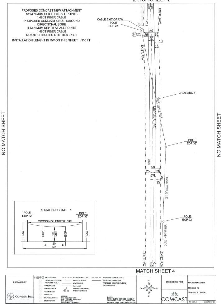
NOTES: BORE HOLE TO BE FILLED SAME DAY VAULT HOLE TO BE FILLED SAME DAY ALL HOLE TO BE TAMPED AND SODDE
